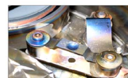
Source boat: W, Mo → high melting point (ca 3000K)
