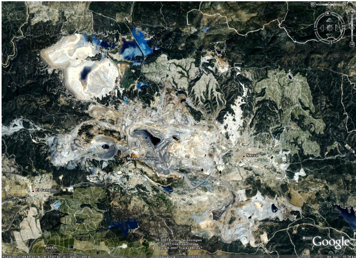
Figure 1.3. Satellite picture of the Rio Tinto mine area. Corta Atalaya pit can be observed in the mid-left part of the picture. White-to-gray areas are mine-weathered extensions of land in the search for iron ore, copper, silver and other mineral ores
