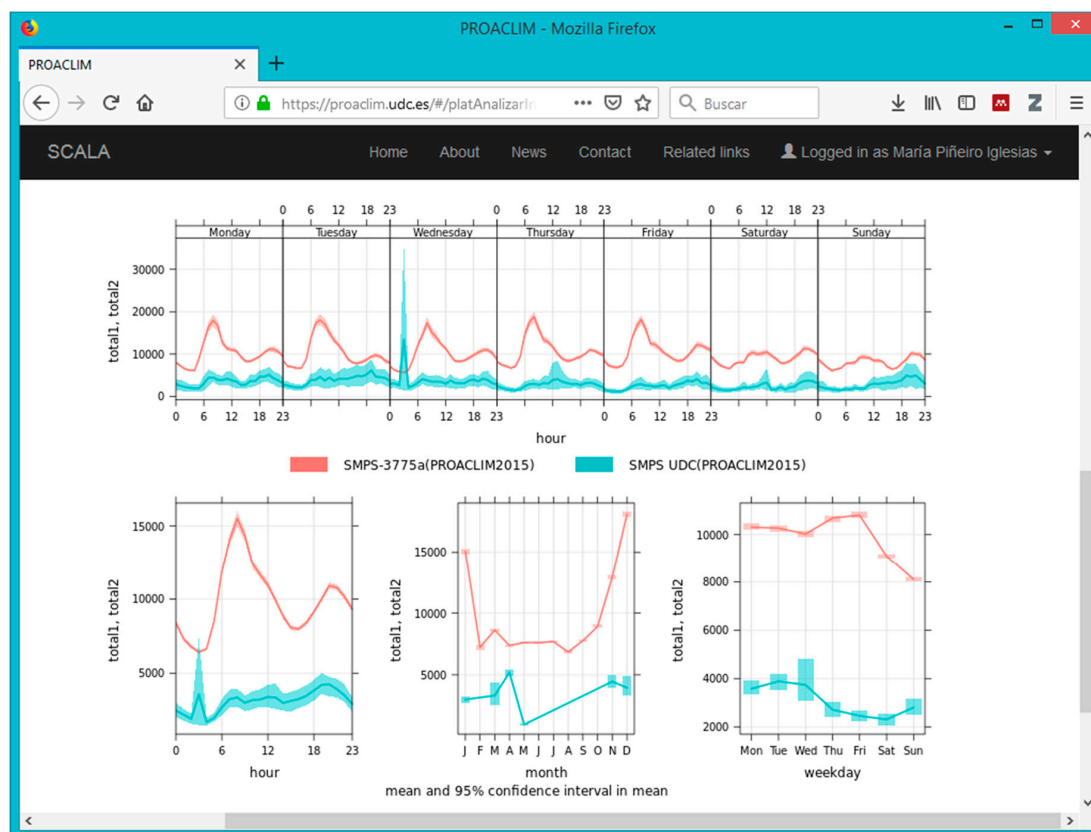
Figure 8. Total particle number concentration ( \text{cm}^{-3} ) vs. time (UTC hour, month and day) for the year 2015 at CIEMAT (total1) and UDC (total2) sites.
