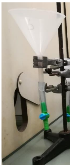
Figure 8 – Density separator system used in this study. The system consisted in a glass funnel fitted with a latex tube on the bottom of the stem and a faucet to control de liquid flow.
