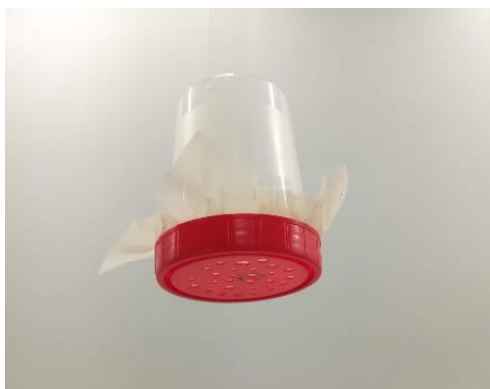
Figure 9 – System created and used in this work to wash the mesh with the MPs; consists in an open flask and holes in the lid, the mesh is immobilized between the flask and the lid.
