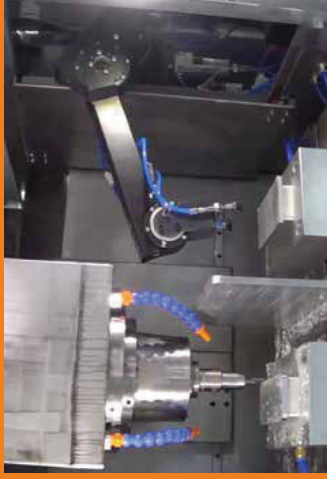
robolink® D – Suction arm in a machine tool (igus®)
