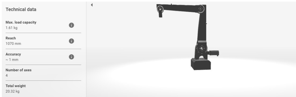
Figure 204 - Configuration of the robolink-type D from igus [136].
