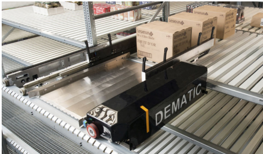
Figure 58 - Dematic Multishuttle® equipped with a telescopic load extractor [30].
