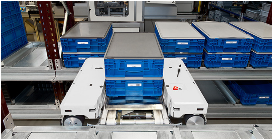
Figure 61 - YLOG-shuttle-system (from KNAPP AG) with an extractor plate that moves over a belt conveyor [112].
