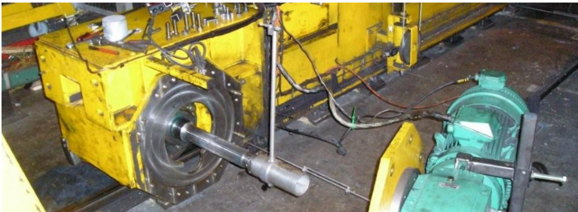
Figure 54 - Maintenance of the gearmotor of a stacker crane [110].
