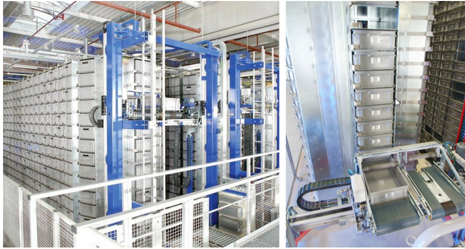
Figure 27 - Lifting system for the carousel AS/RS. Adapted from [34].
