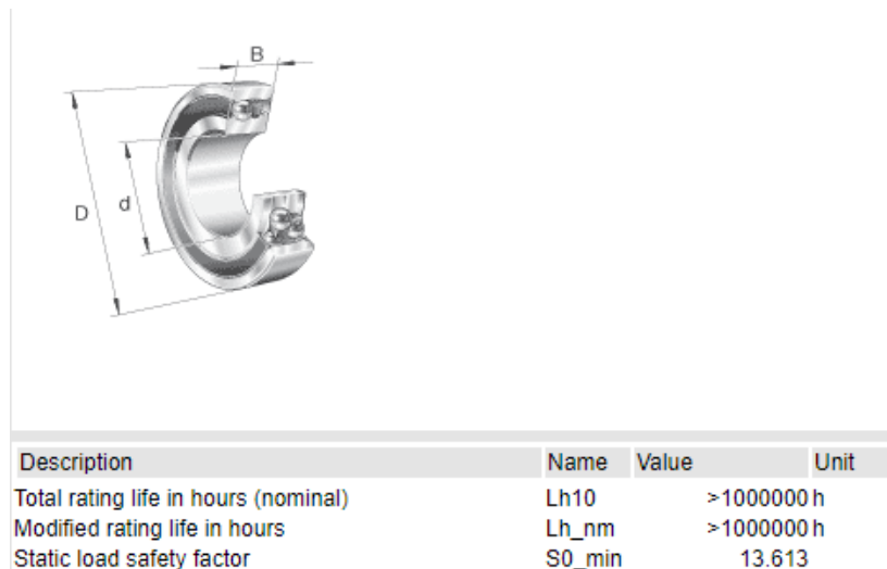
Figure 165 - Schaeffler website - Calculation of the driving shaft bearings from the extraction system – Rating life and safety factors for the bearing.
