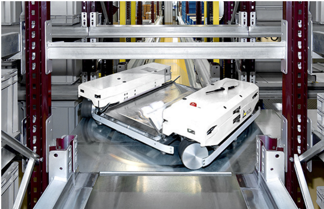
Figure 62 - YLOG-shuttle-system (from KNAPP AG): pivoting wheels that allows the vehicle to move transversely and longitudinally [112].
