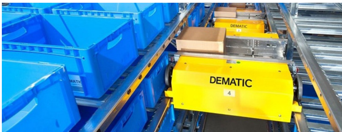
Figure 57 - Example of a shuttle vehicle for cartons, totes or trays [68].
