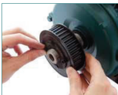
TIGHTEN SCREWS FINGER TIGHT
