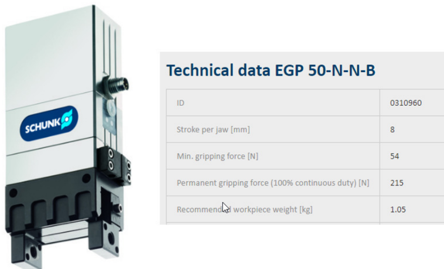
Figure 206 – Selected gripper from Schunk and the main technical data. Adapted from [137].
