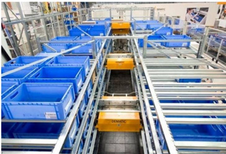
Figure 24 - Box shuttle AS/RS [31].
