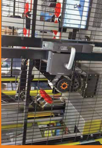
Injection-moulding process with automated handling thanks to robolink® D with 4 DOF (Dr. BOY GmbH & Co. KG)
