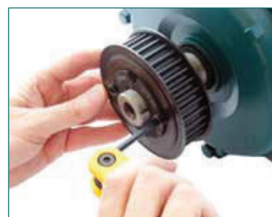
TIGHTEN SCREWS ALTERNATELY
