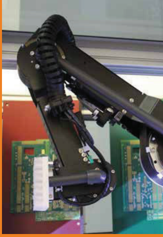
robolink® D for checking printed circuit boards (4Stars Engineering Systems GmbH)
