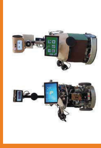
"HOBbit" service robotics project at TU Vienna. robolink® articulated joints on autonomous systems. (Project partner Hella Automation, Austria)
