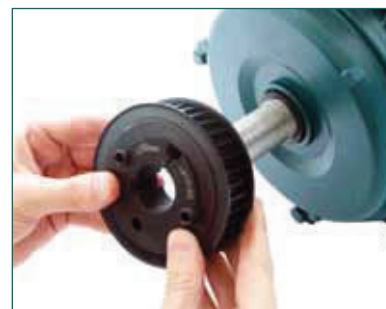
INSERT SCREWS AND LOCATE ON SHAFT
