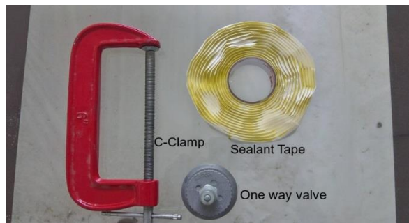
Figure 63 Clamp, sealant tape, and valve
