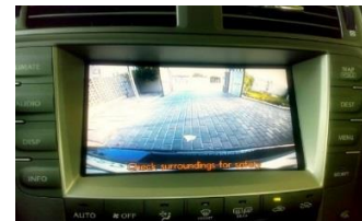
Figure 8- Rear view camera [8]
