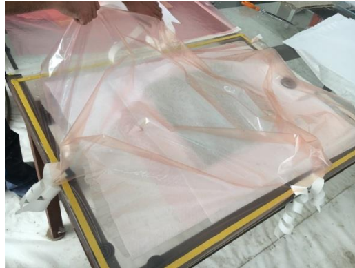
Figure 58 Setting up vacuum bagging
