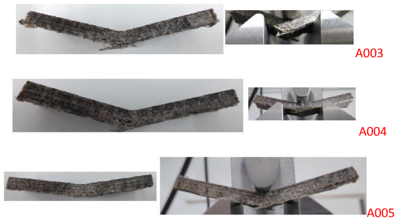
Figure 81 Failure mode view of specimen A
