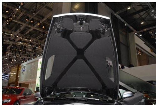
Figure 37 Aston Martin V12 Vanquish inner CFRP hood [107]
