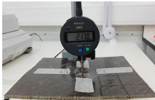
Figure 89 Impact indentation measurement
