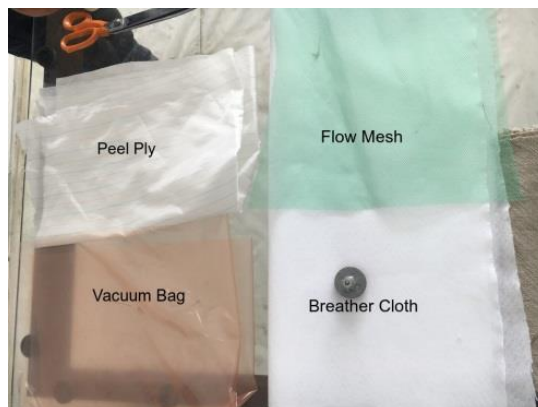
Figure 61 Peel ply, flow mesh, vacuum bag, breather cloth
