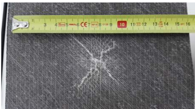
Figure 89 Impact indentation measurement
