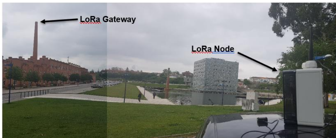
Figure 6.2 – LoRa Gateway (left), at an height of 30m and LoRa Node placed in a car (right), at an height of 1.5m from the ground
