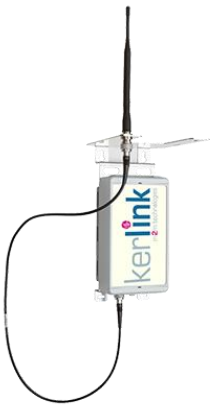
Figure 4.10 a) – MCG (Kerlink IoT Station with SX1301 embutted)
