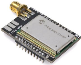
Figure 4.10 b) – SCG (RN2483 module with SX1272 embutted)
