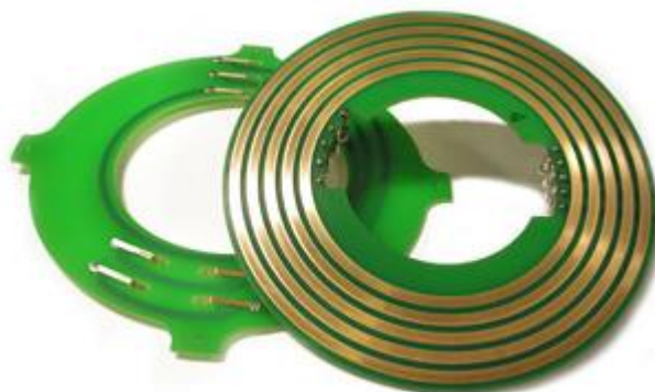
Figure 3 – Example of a pancake slip ring that can be used in a mechanical rotary encoder.
