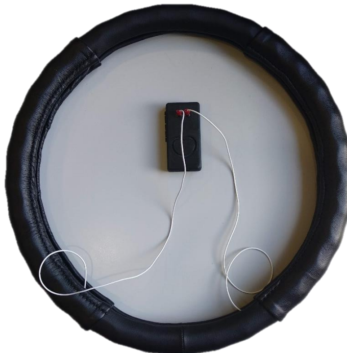
Figure 23 – Conductive leather cover for the steering wheel with the electrodes placed on it.
