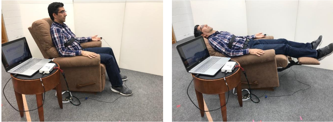
Figure 3.6: Two chair positions were tested in the study: Upright (left) and Reclined (right). For ground truth reference, a chest band and a finger pulse transducer were worn by each study participant.
