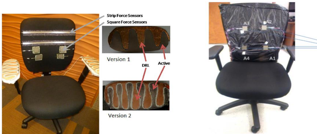
Figure 2.1: Chair sensors used in the related work, that involve placing sensors on the armrest (left) [14] and the backrest of the chair (right) [31].
