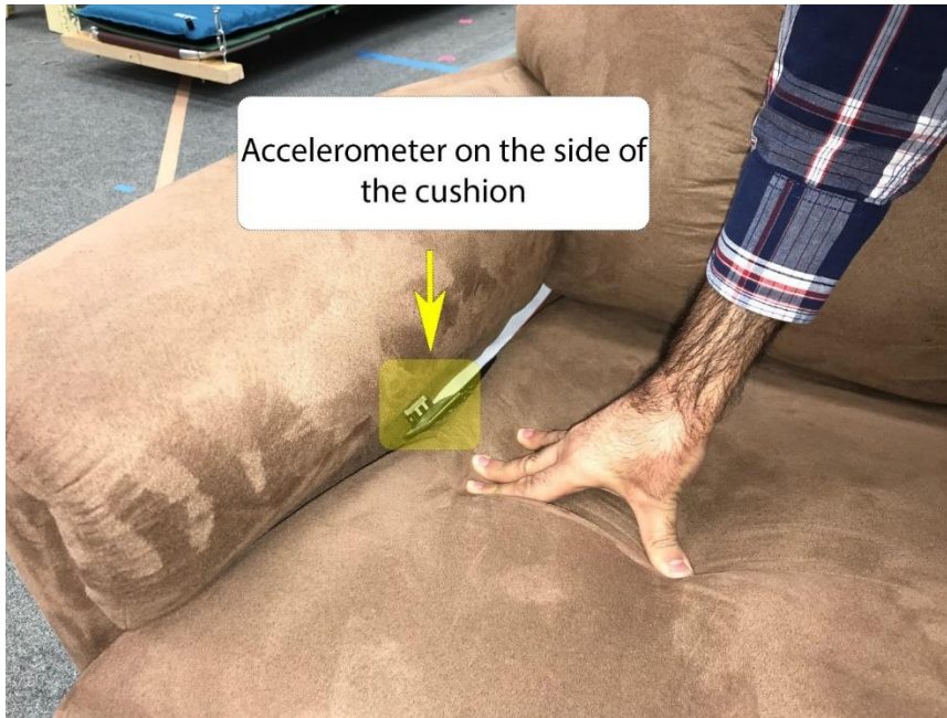
Figure 3.1: Accelerometer placed on the side of the seat cushion, hidden between the seat cushion and the arm of the chair
