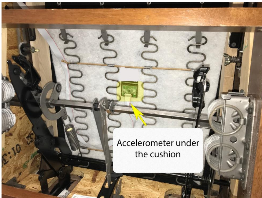
Figure 3.2: Accelerometer placed under the seat cushion of the Recliner chair
