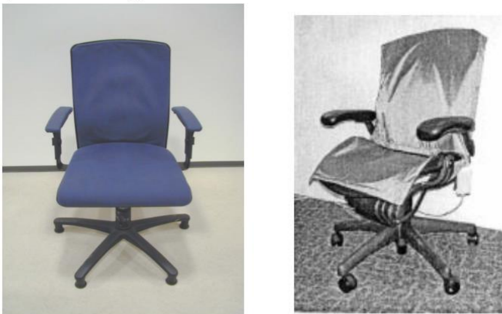
Figure 2.2: Chair sensors used in the related work, that involve placing an EMFi film on the seat and backrest (left) [14] and a pressure sensor mat (right) [22].
