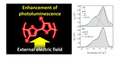
Enhancement of photoluminescence of P3HT dispersed in a PMMA film induced by application of electric field, as a quadratic field effect
