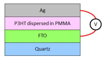
Fig. 1. Layer structure of the device used in the present work. FTO and Ag films were used as electrodes to apply external voltages (V) to the P3HT dispersed in a PMMA matrix.
