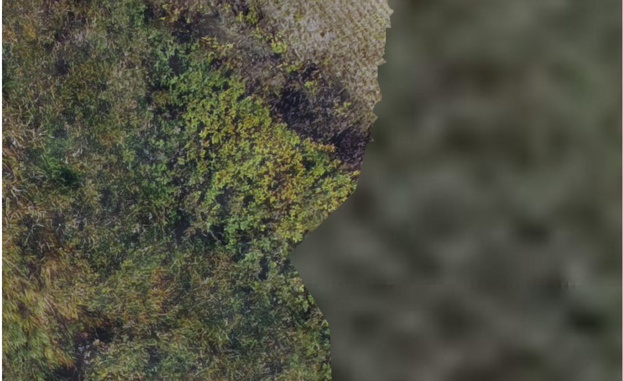
Figure 4-29 Resolution comparison between UAV orthophoto and satellite imagery available on Google Earth (1:60 scale)
