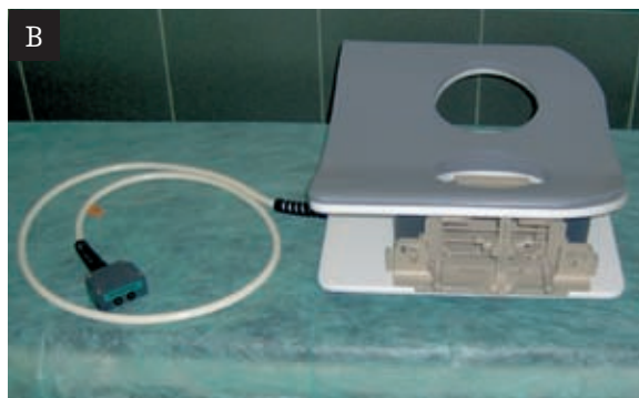
Figure 1. Breast MR coil A. Open breast coil allowing breast biopsy only from lateral access B. Open breast coil with immobilization and biopsy positioning device.
