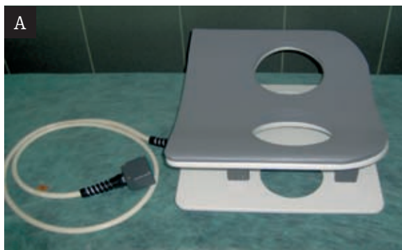
Figure 1. Breast MR coil A. Open breast coil allowing breast biopsy only from lateral access B. Open breast coil with immobilization and biopsy positioning device.
