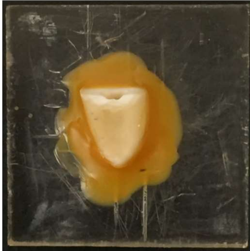
FIGURE 5. Sectioned root mounted on acrylic plates using sticky wax.
