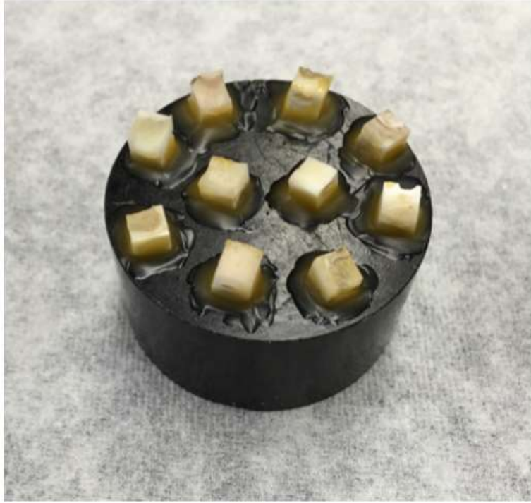
FIGURE 7. 4x4-mm dentin samples mounted on polishing jig.
