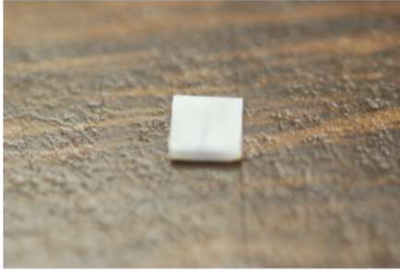
FIGURE 9. Example of polished 4x4-mm dentin sample.
