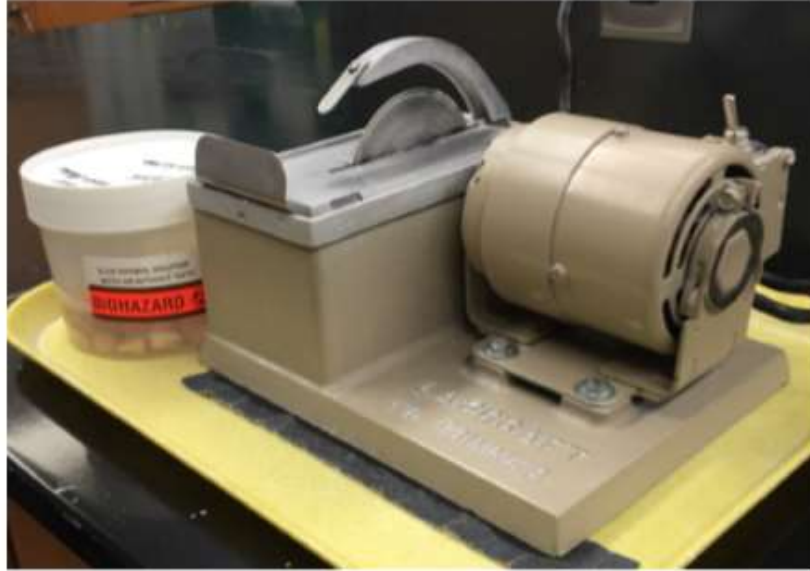
FIGURE 4. High-speed saw used to initially section whole teeth.
