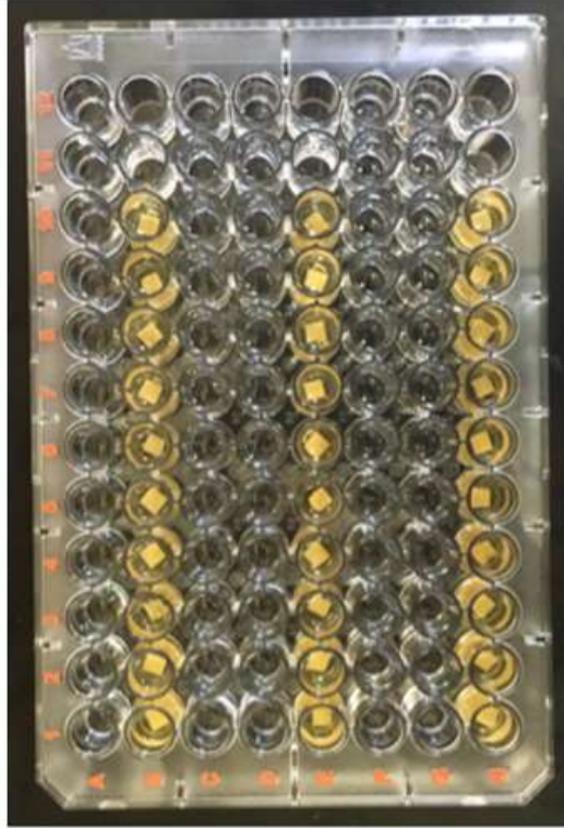
FIGURE 12. Inoculated dentin specimens with BHI-YE broth.
