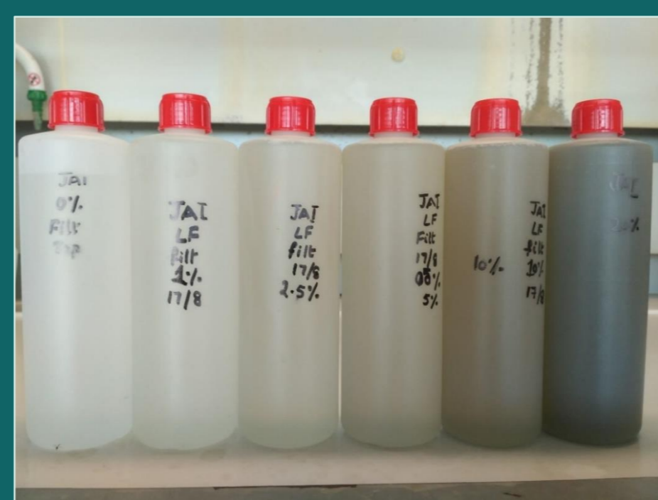
Fig 2 : Series of 0-20% v/v samples of paper filtered liquid fraction of digestate. For eg. 10% v/v = 10x diluted with filtered tap water
