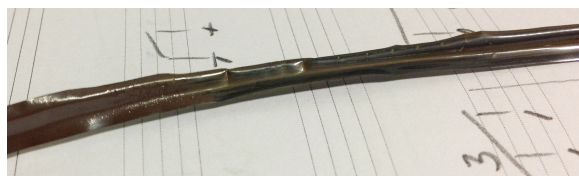
Fig. 4: Example of tape damaged during replay on a machine with bad breaks.
