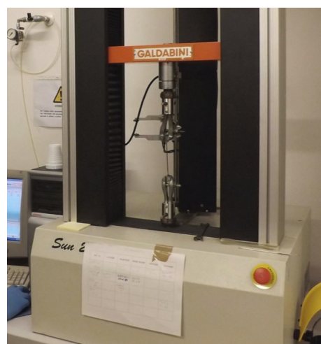
Fig. 1: The instrument used for the tensile test: a dynamometer Galdabini SUN2500 with a load cell of 25,000N.
