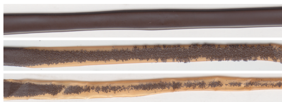
Fig. 3: Different degrees of deformation of a magnetic tape during a tensile test.
