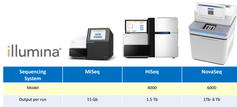
Figure 1.2 This figure compares the throughput of three popular Illumina machines (MiSeq, HiSeq and NovaSeq)
