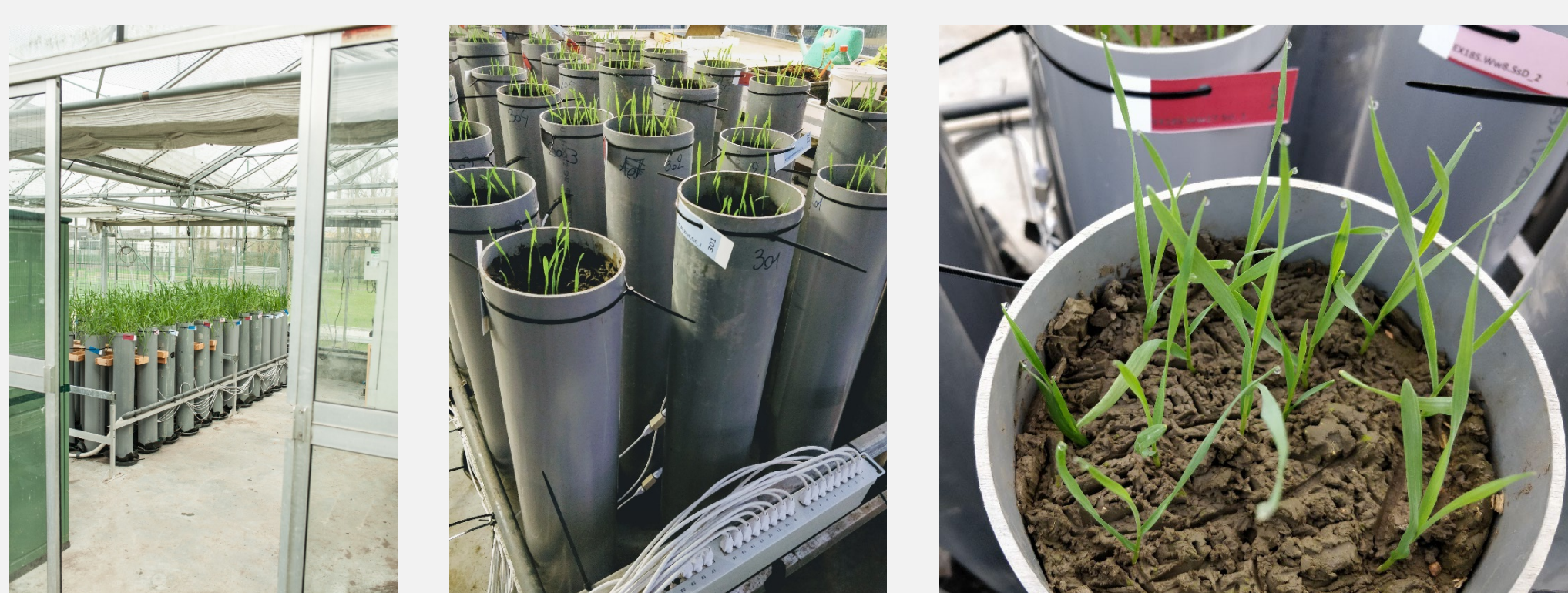
Fig. 1: setup of the greenhouse trial with tailor-made soil moisture registration system
