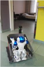
Figure 2: Front and backside view of the platform used by the social robot to move efficiently through the nursing home. The robot can autonomously step on and off the platform.
