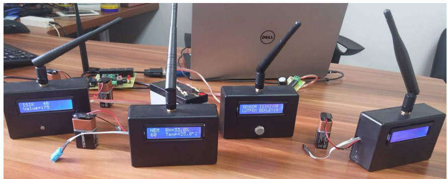
Figure 3. Overview of the designed WSN platform.
