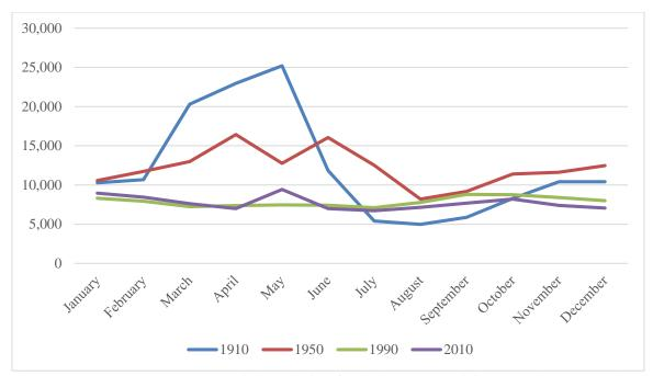
Figure 3.7 Monthly mean cfs (cubic feet/sec) discharge of Snake River near King Hill, Idaho (USGS National Water Information System 2018)
