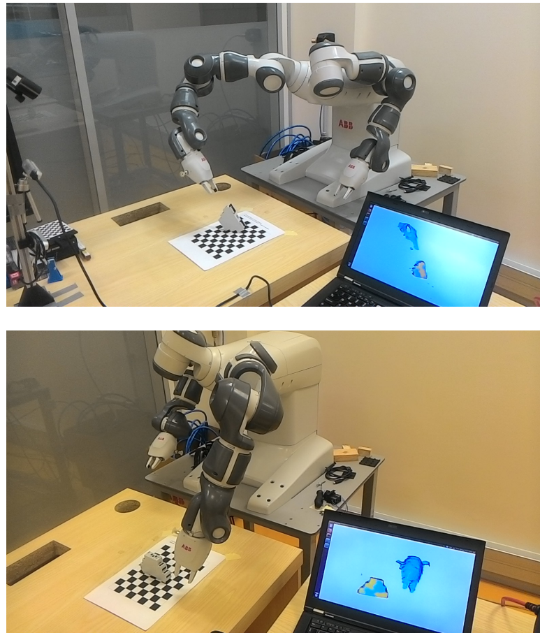
Figure 6.25: Overview 2: Pose Estimation System with the RealSense D-415 Camera.
