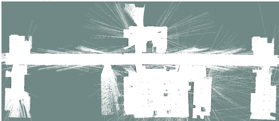
(b) : The Occupancy grid map created by the Gmapping package.
