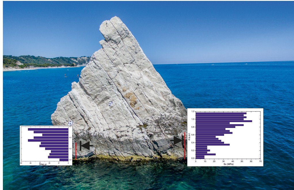
FIG. 10 - Vela seastacks. Lower hemisphere equal area stereonet of the main discontinuities planes: bedding (blue continuous line), joints systems J1, J2, J3 (orange continuous line); joints J4 and J5 with fractures Sz (green dashed lines). In the lower part, values of the uniaxial compressive strength (UCS) estimated with Schmidt hammer apparatus type L (impact energy of 0.735 Nm), respect the distance from the local sea level. The direction of impact with the rock wall is indicate.
