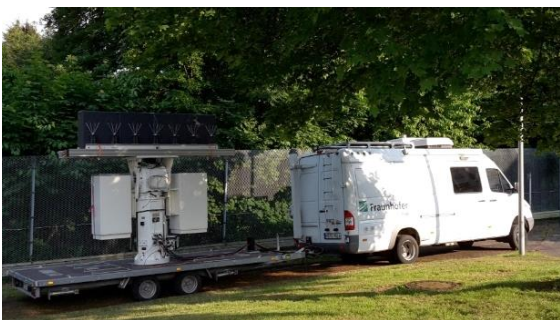
Fig. 3. Multichannel PCL receiver mounted on the back of a van in a side-looking configuration.
