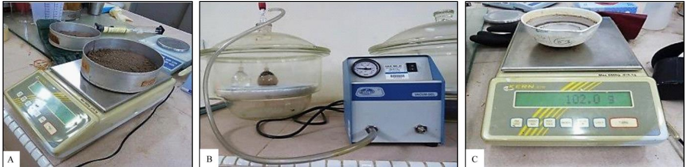
Figure 7 Soil analysis setup (A: weighing of soil sample, B: bulk density determinations, and C: soil particle determinations)
