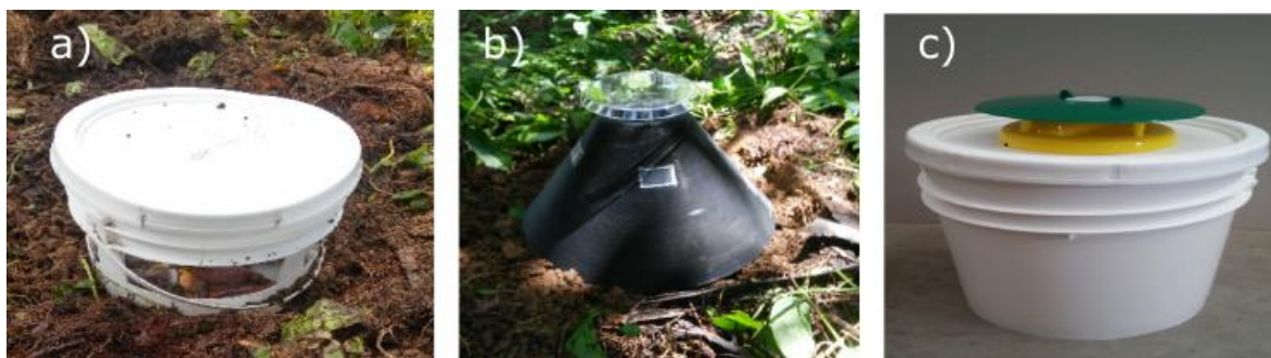
Figure 1. Different trap designs compared for mass trapping of weevils: (A) standard bucket trap with lateral entrances, (B) Electrap TM and (C) modified standard bucket trap with single cone entry point on lid.
