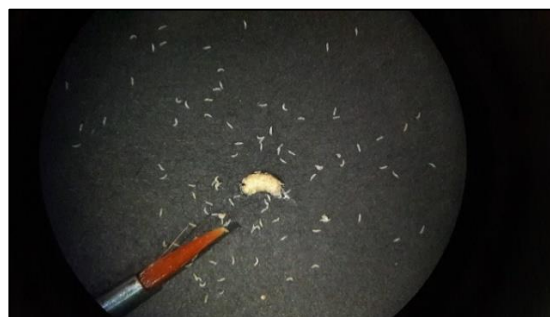
Figure 2. Billaea claripalpis ovary with emerging planidia and brush for transfer of planidia onto a host for host suitability testing
