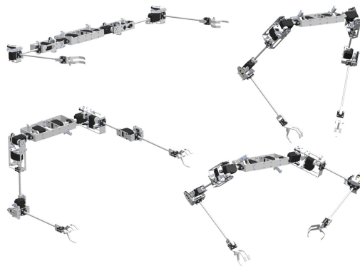
Fig. 2. Different poses of the anthropomorphic dual arm.
