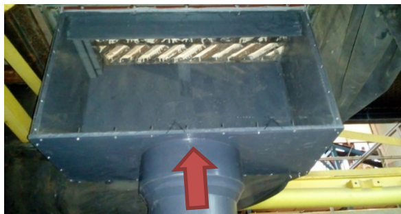
Figure 4:2 Inlet box below the grate.
