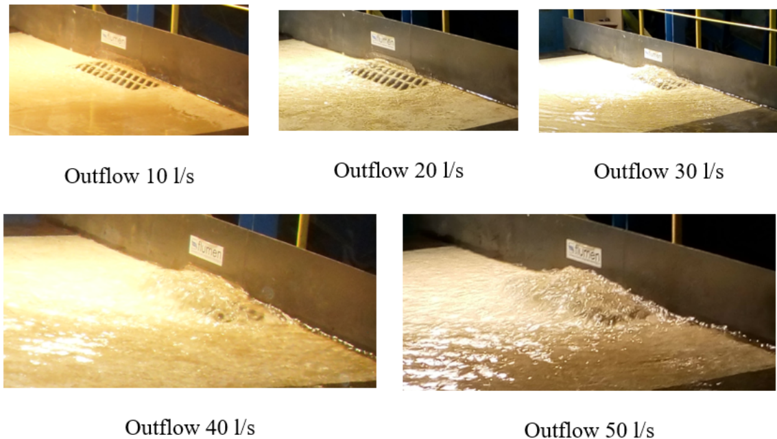
Figure 4:7 Outflow between 10 and 50 l/s for a geometric configuration of the platform with 2% of longitudinal and transverse slopes.
