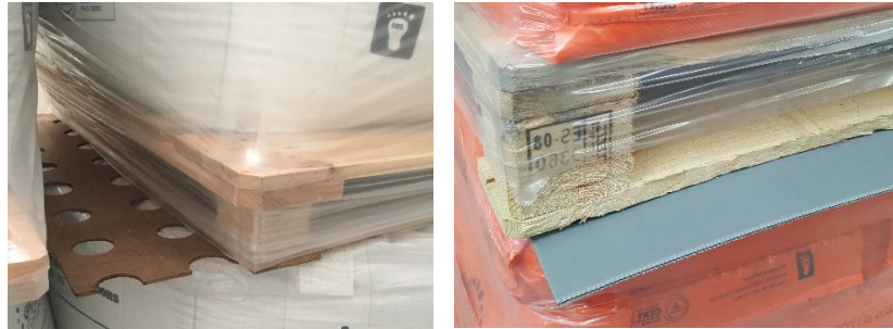
Figure 3.1. Eucalyptus wood sheet (on the left), plastic compound sheet (on the right)
