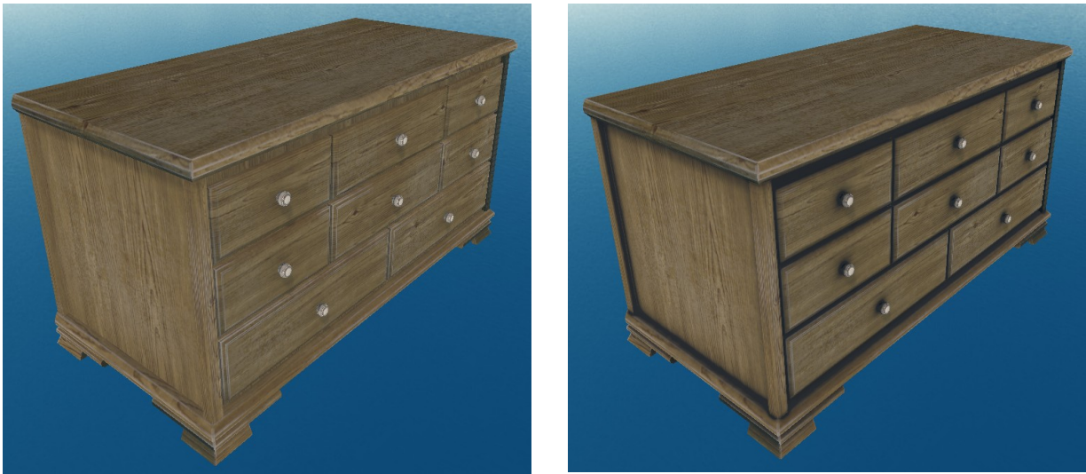
Figure 101: Baking the ambient occlusion into the model color. Left without bake, right with bake. Notice that occluded zones are darker in the picture on the right.
