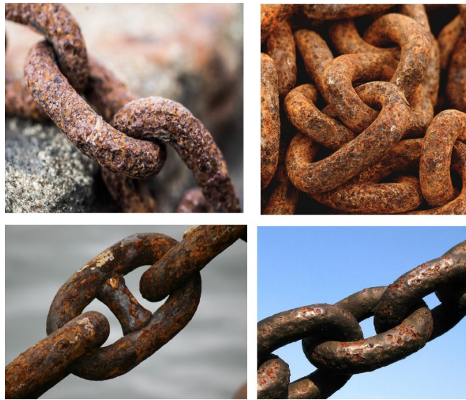
Figure 114: Real pictures of corrosion on chains.
