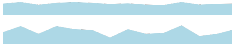
Figure 38: Surface microfacets. Above, a considerably smooth surface. Below, a quite rough surface.
