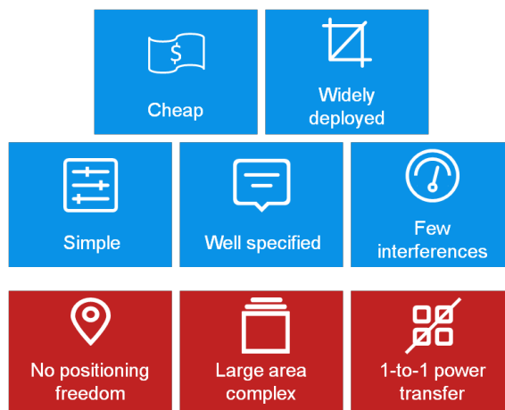
Figure 2.5: Inductive coupling features(blue) and limitations(red)
