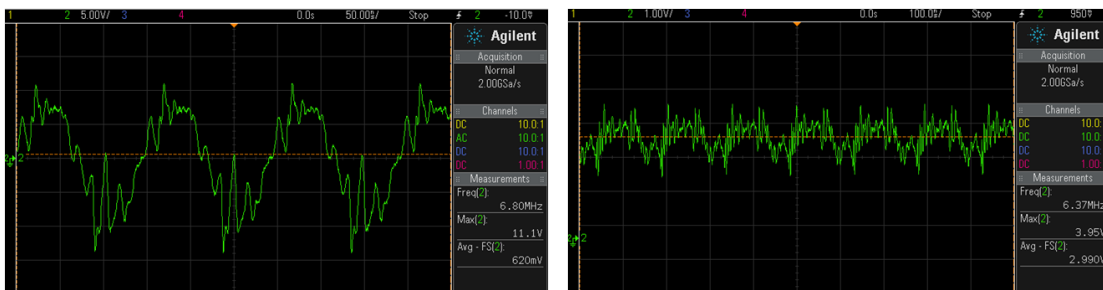
(a) Induced voltage on the secondary winding of the current sensing transformer (b) Rectified voltage after being scaled through a voltage divider
