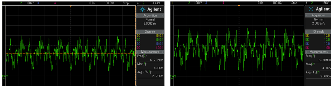
(a) Current sensor regulated output voltage with no receiver (b) Current sensor regulated output voltage with receiver
