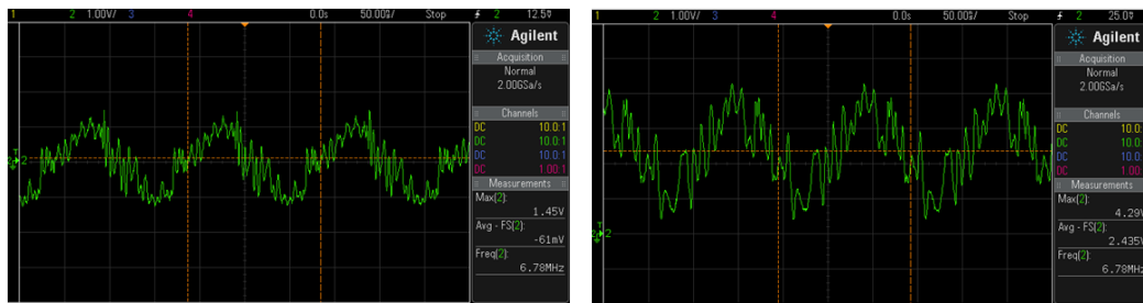
(a) Sensed voltage signal after being scaled down by a voltage divider (b) Voltage measured by the MCU after rectification and regulation stages
