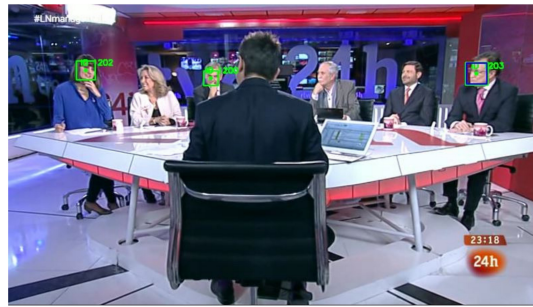
Figure 4.3: The blue boxes represent the detections without upsampling and the green ones with upsampling. The line below each frame represent the final results obtained by the system. The last two fields are the name of the person and the track ID that we can also see it in the image. In the first frame, the detector with upsampling detects two more faces than without upsampling, but for example the track 116 is wrongly identified because that woman is not Julio Somoano. Similar things happens with the track 425 in the second image and the track 1200 in the third one. All of these three cases have faces in odd positions that we detect only with the upsampling step, but are wrongly identified.
