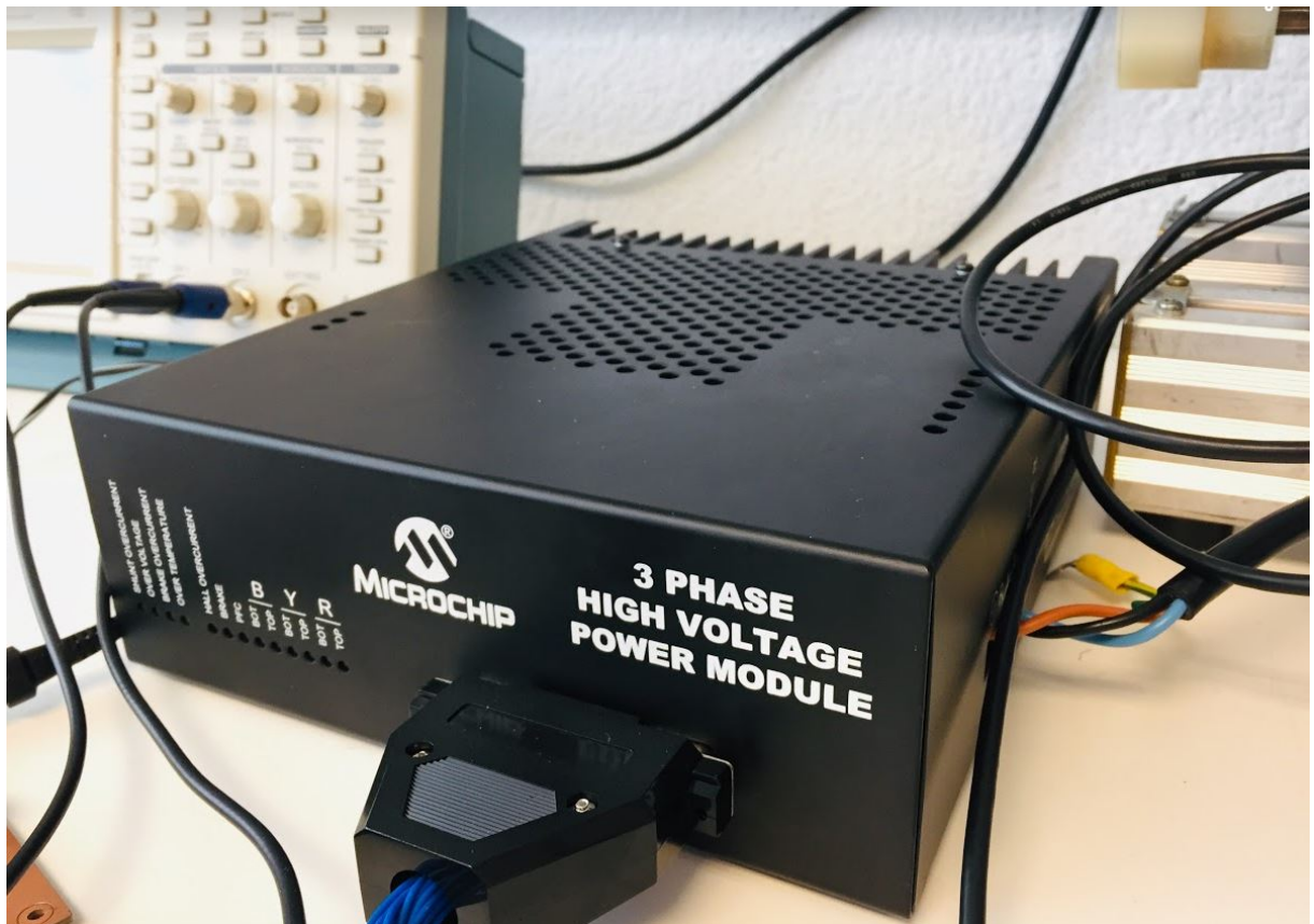
Figure 7.3 3-Phase High Voltage Power Module MC1H Inverter
