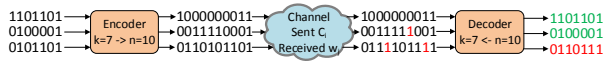
Fig. 6. Three different messages are encoded by the codebook constructed with MIP for t_s = 400 ms, M = 400 , (n, k) = (10, 7) .
