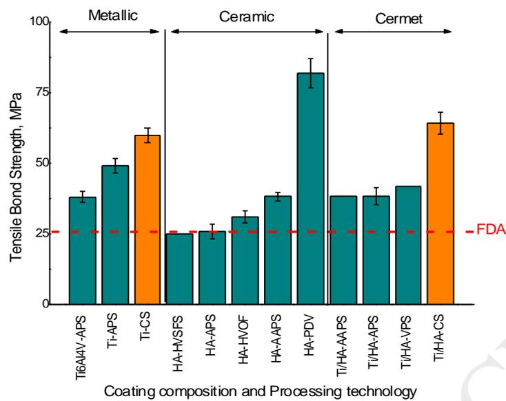
**Figure 4.** Tensile Bond strength values of coatings (metallic, ceramic and cermet) produced by different technologies including the CGS coatings produced in this study (highlighted in orange). Values in green were obtained from the literature [27,58,60,62,88–90].
