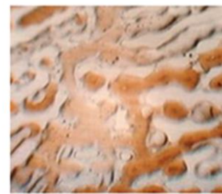
Stage-3: CO 2 has developed miscibility with oil at 17.2 MPa and 315 K (above MMP). The miscible fluid is very dilute (light) flowing in the pore channels
