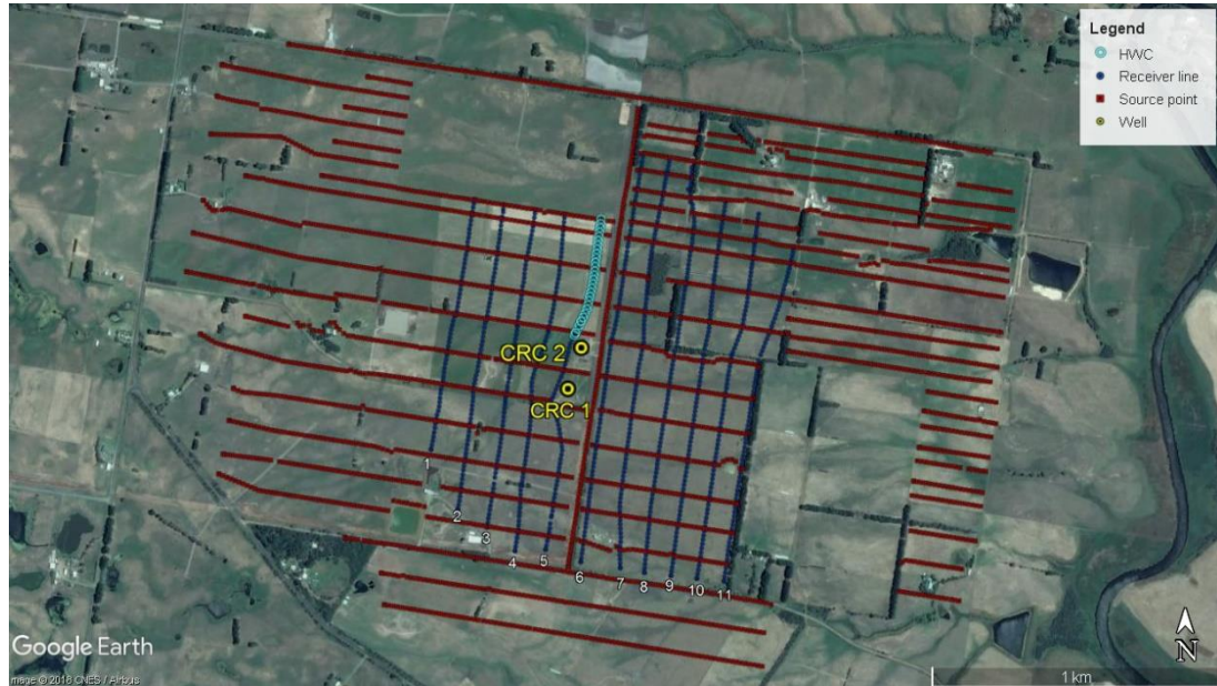
Figure 5.3 Acquisition design at the Otway site: receiver lines (blue), shot points (red).
