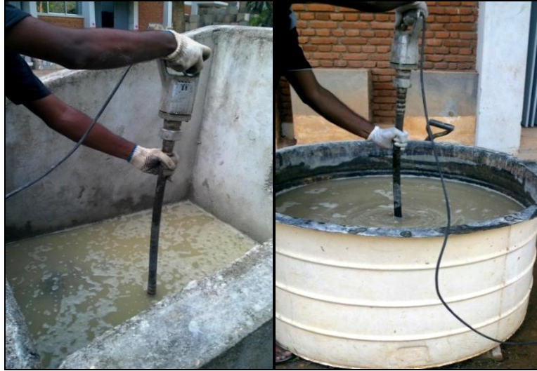
Figure 1. Application of poker vibrator in both circular and square containers, under saturated condition
