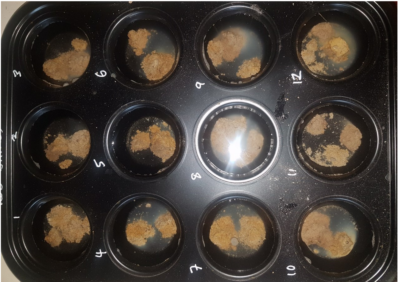
Figure 5.1: Dispersion in varying pH NPS at 5 min. Sample 1 has pH 4. Subsequent samples have pH rising in increments of 0.2 pH units to sample 12 at pH 6.4. Experiment continued on next tray.
