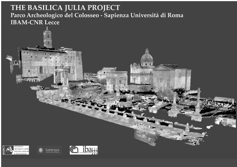
▲ Fig. 1 The point-cloud arising from the architectural survey of the Forum Romanum is integrated with the point-cloud produced image by the survey of the Fabbrini's excavation
