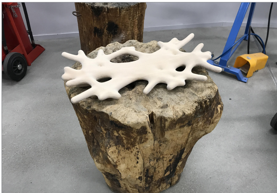
Fig. 49 Seat before manual sanding. Tool paths can still be seen on the surface.
