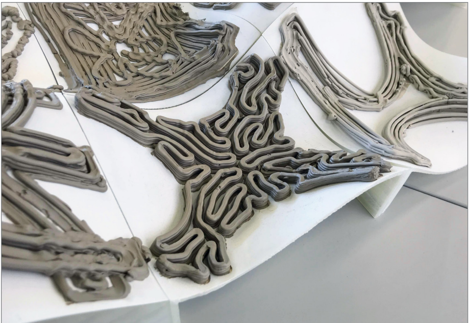
Fig. 19 Robotic clay deposition results.
