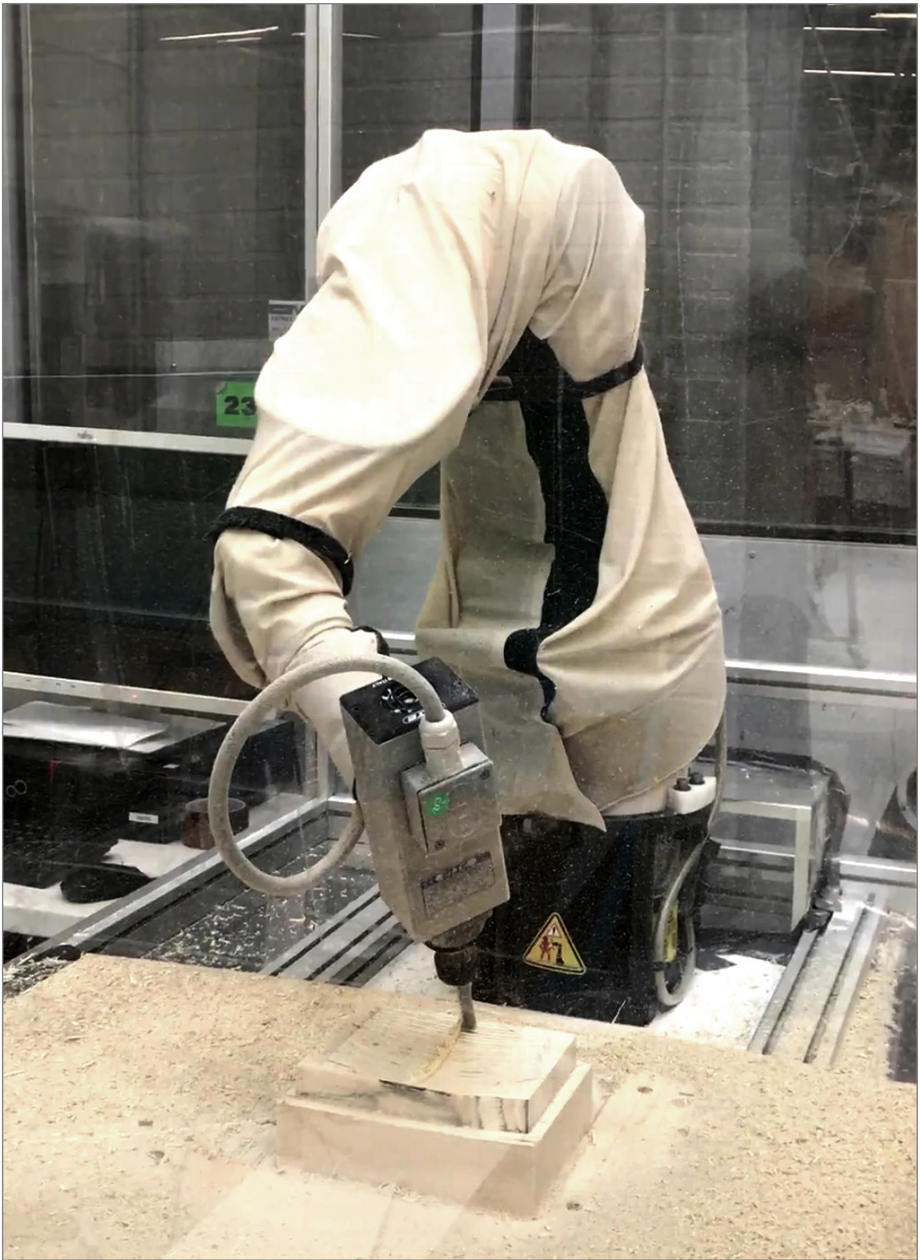
Fig. 16 Early testing of KUKA|prc plug-in for Grasshopper at Aalto University Digital Design Laboratory. A robotic arm mills a block of Laminated Veneer Lumber (LVL). A seamless digital process was achieved, from geometry generation to fabrication, all within one software. The exercise proves that the process studied in the thesis is technically viable.
