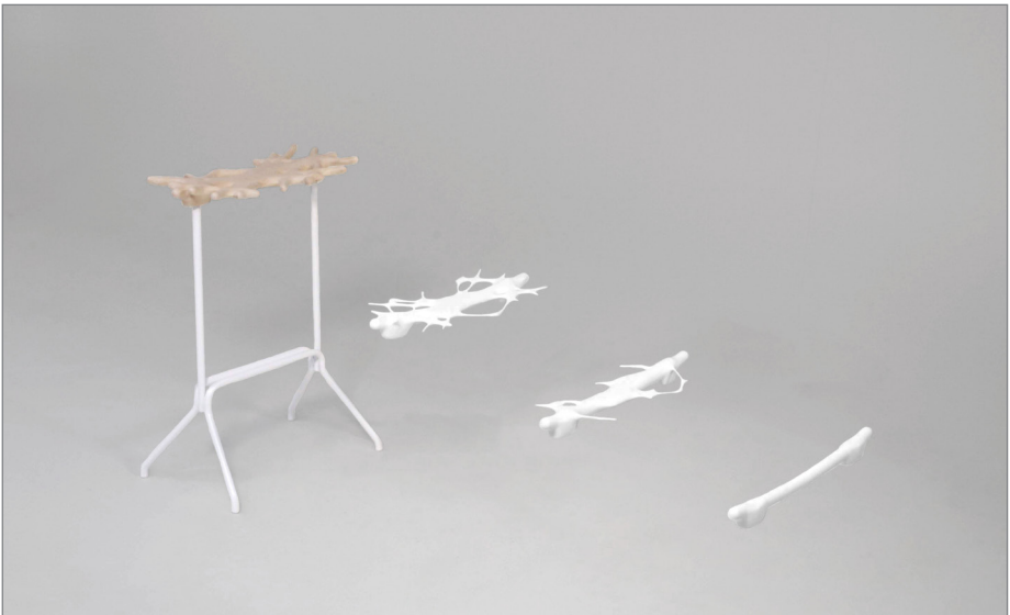
Fig. 54 Form development stages. The initial form contains all elements that remain constant across all iterations; it includes a transversal beam for structural rigidity, pockets for leg structure placement, and added mass for screw connections.
