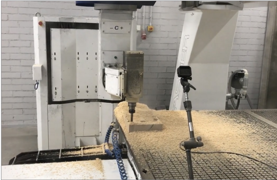
Fig. 46 CNC milling process. A rough pass first removes most of the unnecessary material followed by medium and fine passes that gradually form the seat.
