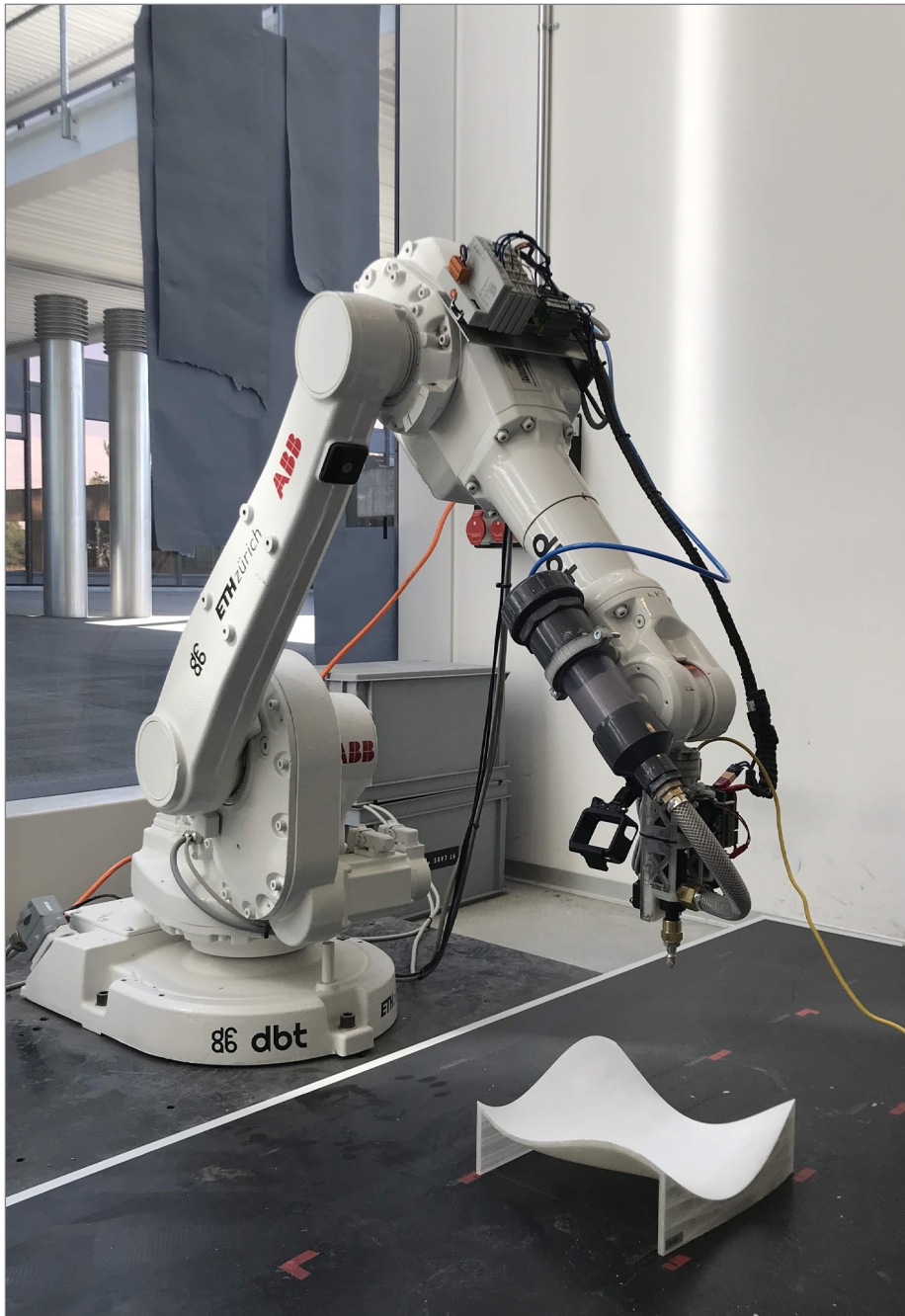
Fig. 17 Robotic arm used during the RobArch workshops in Zurich 2018. The arm was retrofitted with a custom device for controlled clay extrusion.
