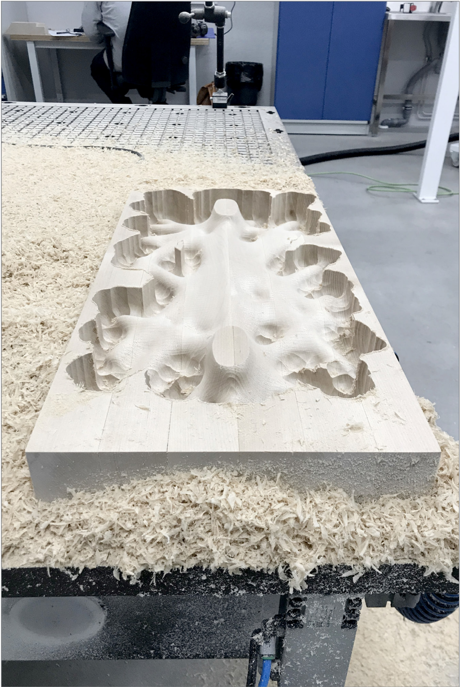
Fig. 48 Bottom side milling complete.
