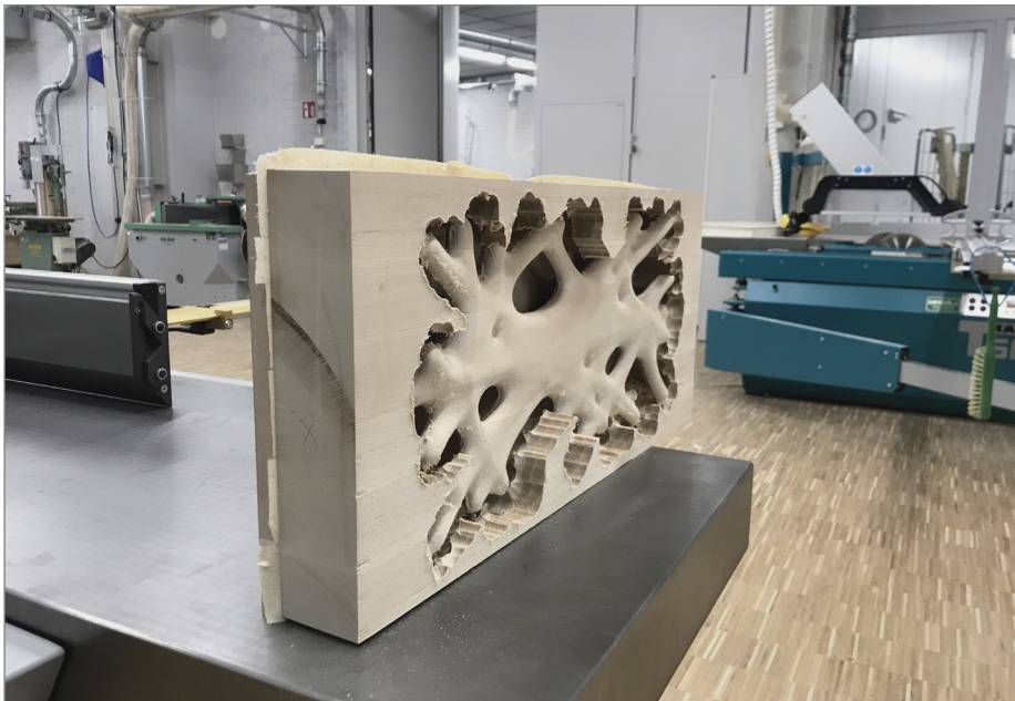
Fig. 47 As the milling is complete, the seat has to be detached from the block.
