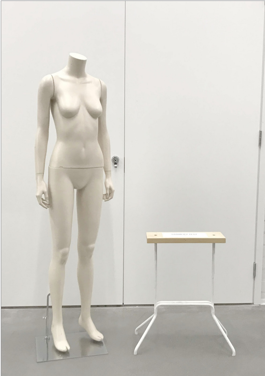
Fig. 42 Structural test of an initial structure design. The connections showed enough strength to withstand the average weight of a user. The leg angle was considered too wide; the next iteration featured tighter angles resulting in improved proportions while maintaining the required structural rigidity and stability.
