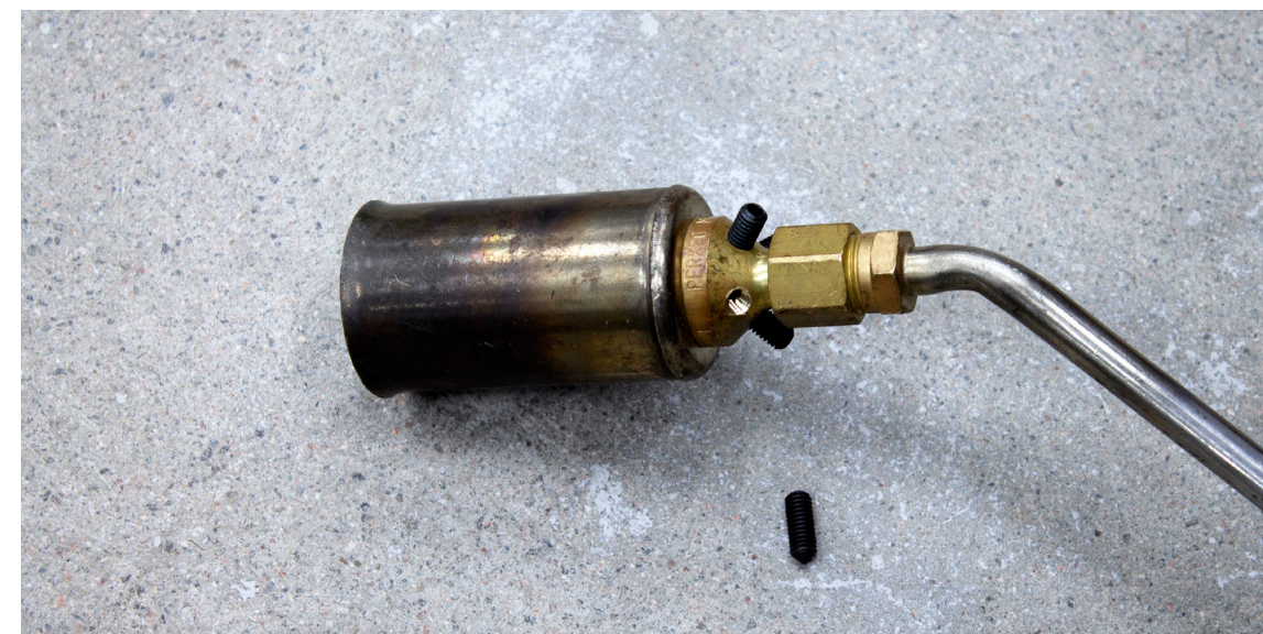
Fig. 24. Modification on hand burner head
