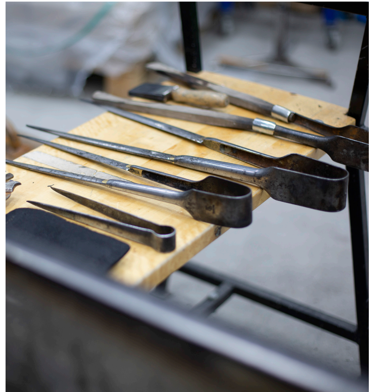
Fig. 28. A view on a collection of different jacks used for my process
