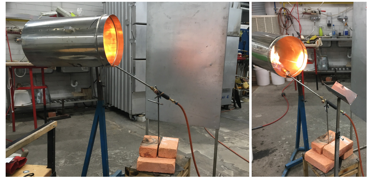
Fig. 64. My flaming chamber design for the reduction process and its variations
