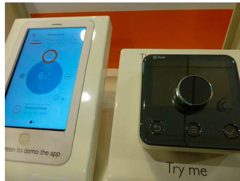
Figure 3. Example of smart heating controls.
