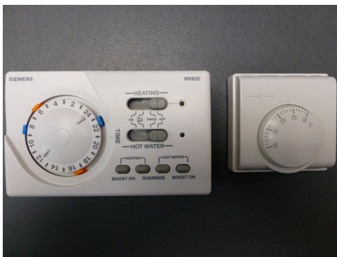
Figure 1. Example of a mechanical thermostat and programmer with 'pins' to manage on-off times. All images are authors' own.
