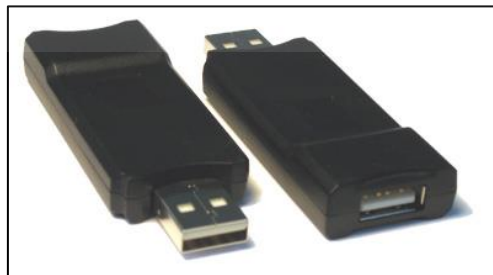
FIGURE 20: IN-LINE USB KEYLOGGER (KEYCARBON LLC, 2017)
