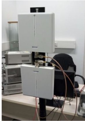
FIGURE 6.8: Set Up for the Bistatic Reflection Mode Calibration
