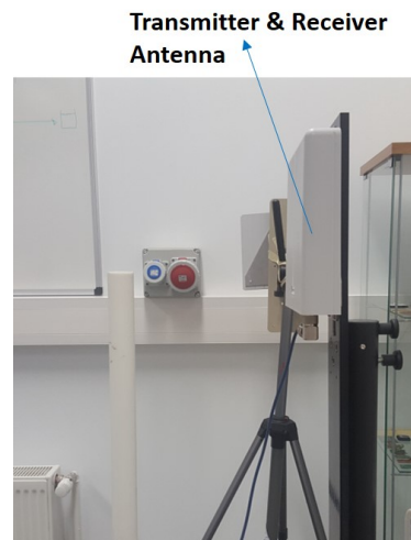
FIGURE 6.11: Set Up for the Monostatic Reflection Mode Calibration
