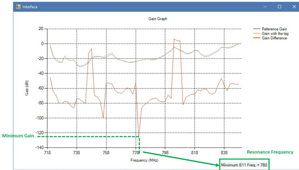
FIGURE 5.22: Plot of the Gain of the S11 and Minimum Identification
