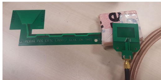
FIGURE 6.27: Set up of Tag 1 for the measurements
