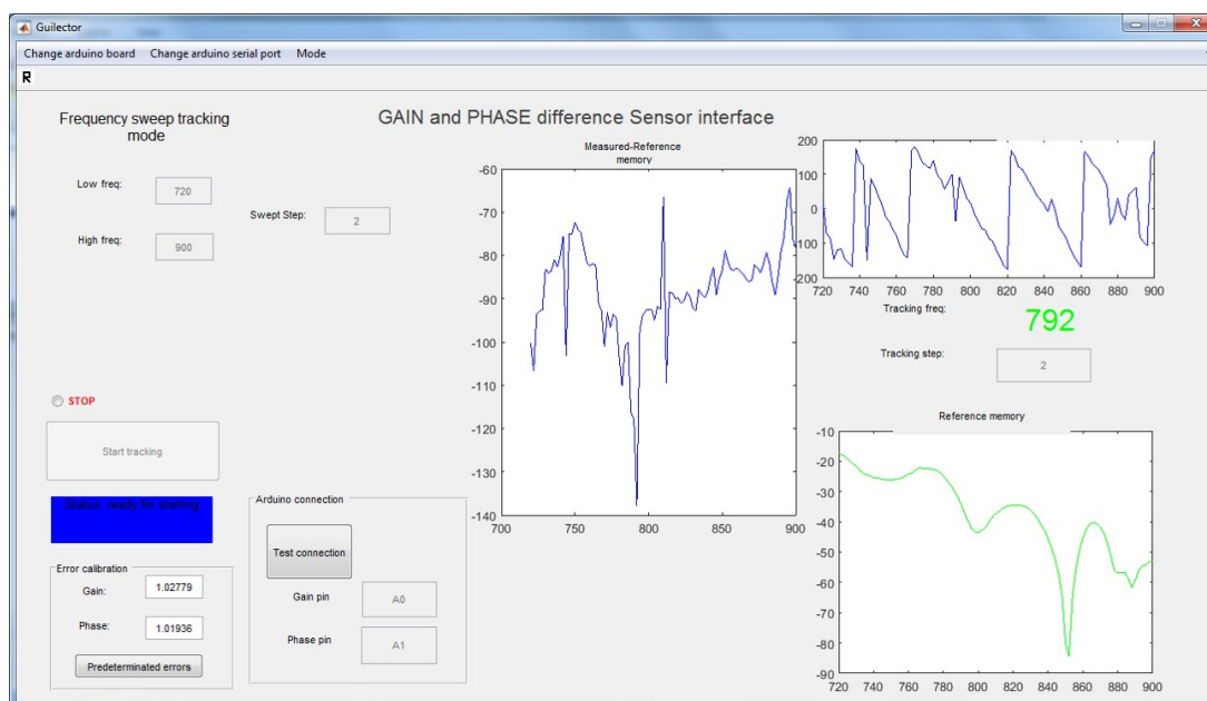
FIGURE 6.14: 780 MHz Tag Monostatic Reflection Mode Measurement
