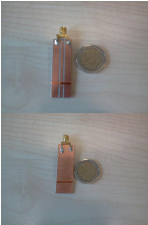
Fig. 3 Target based on a CPW at 868 MHz
