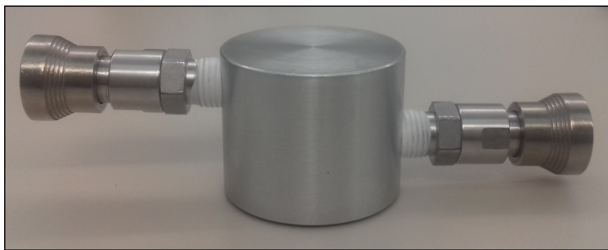
Figure 5.5 – Chamber used to measure the variation in conductivity as a function of the temperature.
