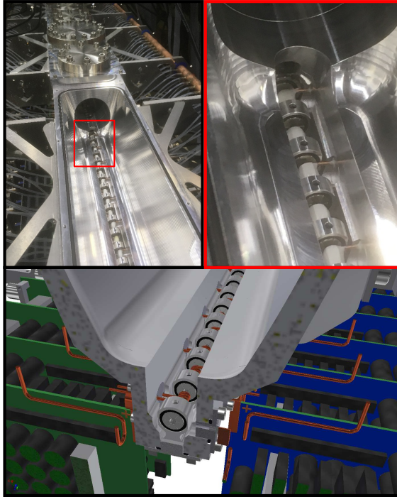
Figure 6.2: Two photographs and a schematic cross-section of the multistage Zeeman decelerator used in this experiment. In the photographs, the lid is removed from the first vacuum chamber. The zoomed-in image shows the connection between two modules, which enables an uninterrupted sequence of solenoids and hexapoles. Solenoids are encased in white epoxy resin (Torr Seal) to resist flexing forces in the solenoids due to self-inductance. The cross-section shows the close proximity of the solenoids and the circuit boards that drive the solenoid currents.
