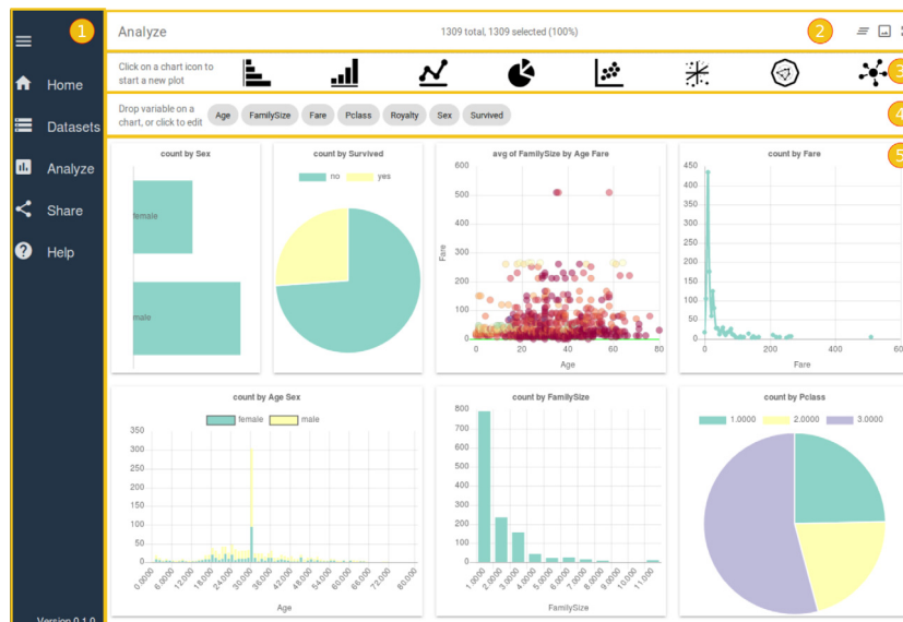
Fig. 3. Web-interface of spot. (1) Main menu: to navigate between different pages. Users can upload data (Datasets page), analyze it (Analyze page), share selection and charts as a session (Share page), and read help documentation (Help page); (2) Information bar: provides basic statistics about selected data; (3) Chart bar: in order to add available charts to the dashboard; (4) Variable bar: lists available variables within the data-set; (5) The dashboard.
