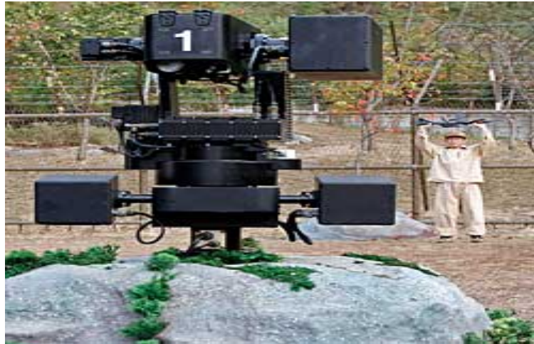
Figure 2.10: A robotic sentry gun developed by Samsung Techwin Co. is shown holding up a potential threat. The SGR-A1 robot uses pattern recognition and object detection based algorithms to identify targets, effectively filtering friend from foe. This is just one such example of object detection being applied to real world technology. Image source [5]
