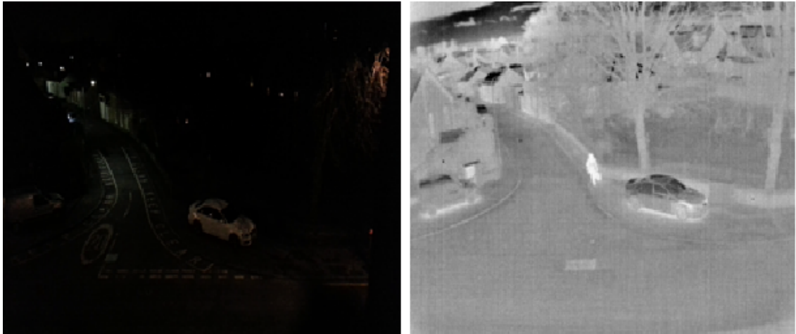
Figure 1.1: The left hand image shows a colour image capturing an urban street scene in Glasgow. Given the poor illumination and sensor band it is hard to discern scene content. The right hand image captures the same view but using a low quality thermal imager, revealing a person in the centre of the scene.
