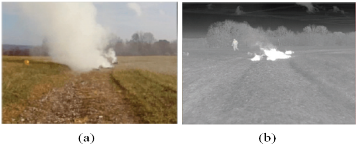
Figure 2.1: Image (a) captures a smoke filled scene using a colour band sensor, where we cannot see anything behind the clutter. Image (b) is a LWIR image of the same scene, where a pedestrian is revealed to be standing behind the column of smoke [1].
