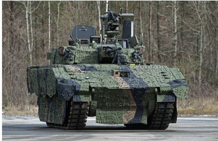
Figure 1.2: The figure presents a prototype Ajax armoured fighting vehicle, soon to be commissioned for use by the British Army. This new breed of vehicle is equipped with state-of-the-art sensors operating in multiple wavebands, as well as local situational awareness systems. One of the key capabilities of the new vehicle design is the electronic architecture and on-board data capture system, as intelligent processing and information analysis is critical to obtain enhanced situation awareness. Image re-used courtesy of ©Crown Copyright.
