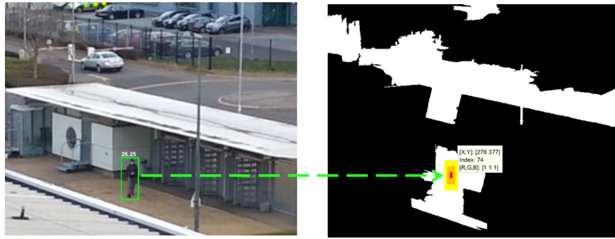
Figure 4.5: Person detection bounding box is mapped to SP variance layer and convolved with Gaussian kernel to aggregate and build confidence map, which is the Foreground-Background layer. The resulting FGBG layer will be utilised to classify thermal signatures without a classifier at a later stage.
