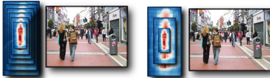
(a) Naive approach for dealing with feature scales. (b) N/K Scales for dealing with feature scales. This is an approximation across scales.
