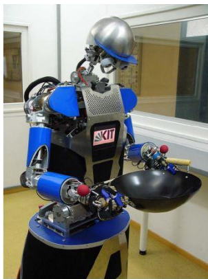
Figura 18: Robot llevando a cabo tarea de manipulación con control visual y ambas manos. Fuente: Vahrenkamp, Nikolaus; Böge, Christian; Welke, Kai; Asfour, Tamim; Walter, Jürgen; Dillman, Rüdiger, Visual Servoing for Dual Arm Motions on a Humanoid Robot, 9th IEEE-RAS International Conference on Humanoid Robots, Humanoids09 (2009).
